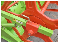
Adjustable Cutter Reel Height for Better Flow of Crop into Burr
