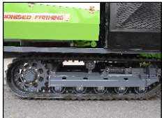
Roller Track Driving Gear. Gearbox special Support Roller with Bridgestone Track.
