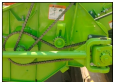
Enhanced Chain Drive System for Better Cleaning
